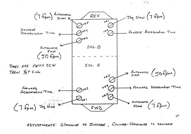
Directional valve used in airless coilines.
